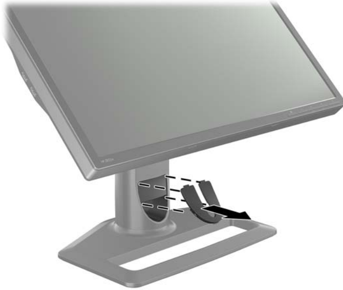
Figure 3-3 Removing the Cable Routing Cover
