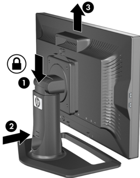
Figure 3-9 Adjusting the Height
