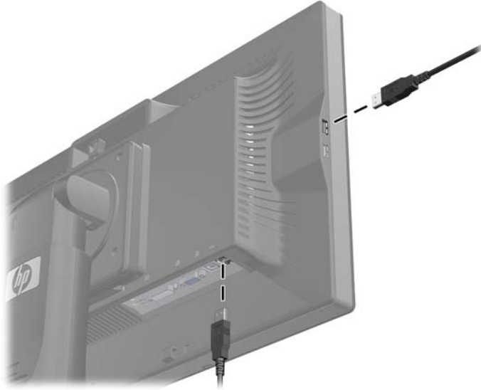
Figure 3-6 Connecting USB Devices
