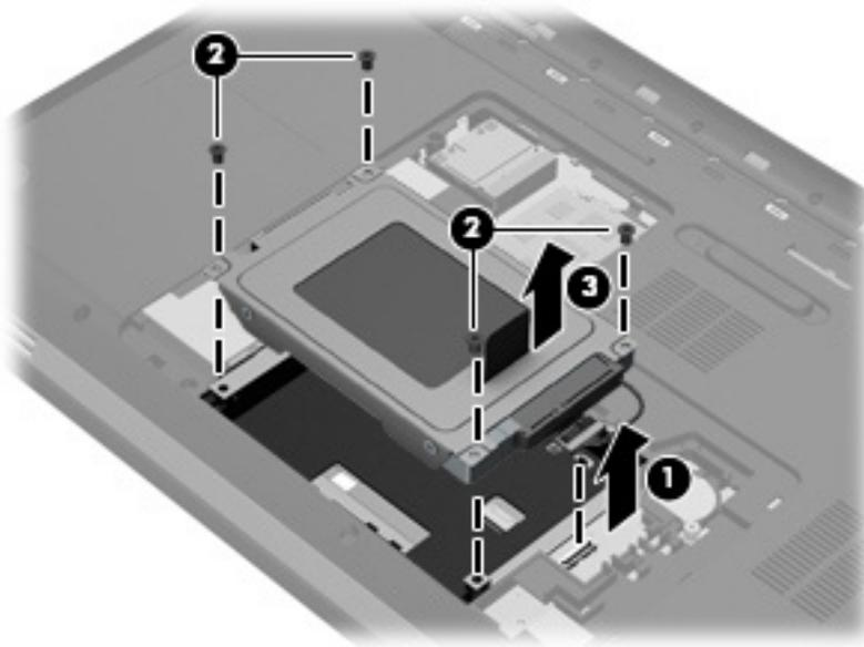
4. If it is necessary to replace the hard drive connector cable or hard drive bracket:
