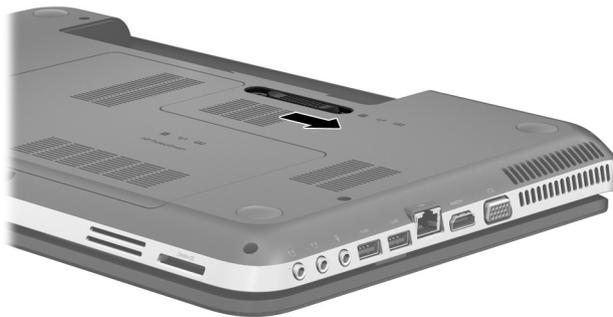
2. Lift the rear edge of the service cover up and forward until it rests at an angle.
