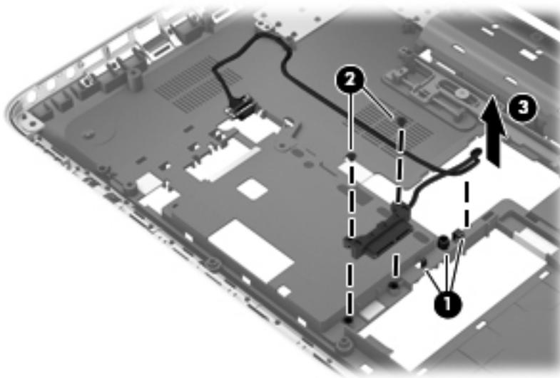
Reverse this procedure to install the optical drive connector cable.
