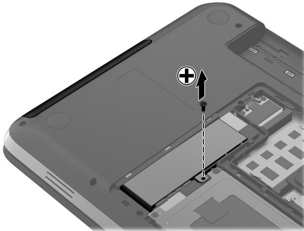
5. Remove the optical drive by sliding it out of the optical drive bay.
