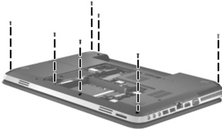
4. Remove the following screws that secure the top cover to the computer:
