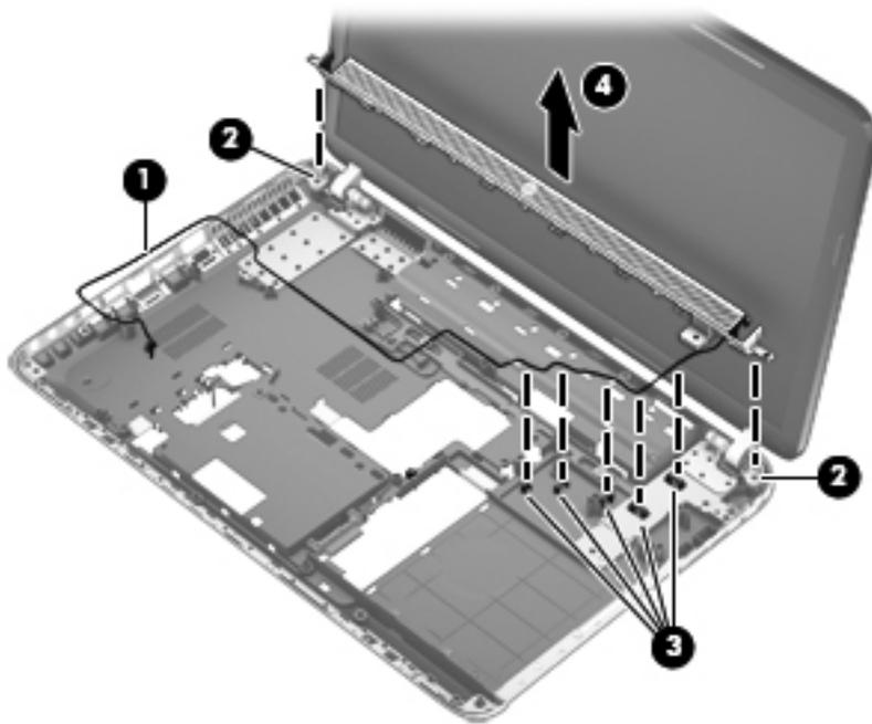
9. Remove the Phillips PM2.5×4.0 screw **(1)** that secures the front speaker to the base enclosure.
