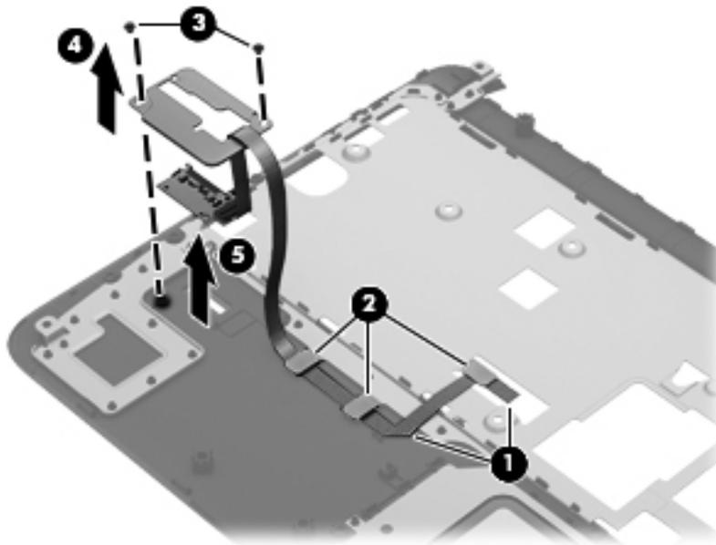
Reverse this procedure to install the fingerprint reader board and cable.
