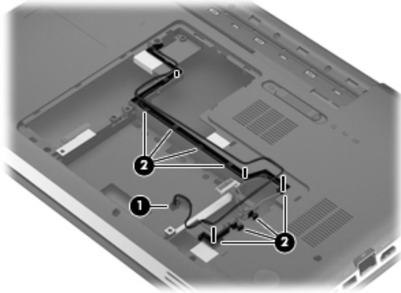
4. Remove the four Phillips PM2.5×4.0 screws **(1)** and the PM2.5×10.0 screw **(2)** that secure the rear speaker to the computer.
