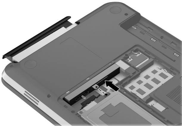
6. If it is necessary to replace the optical drive bracket, position the optical drive with the rear panel toward you.
