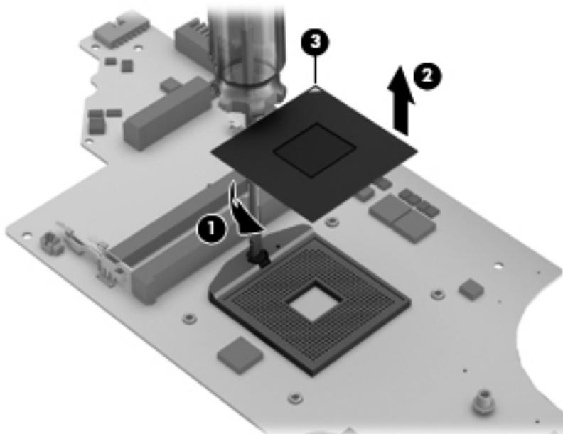
Reverse this procedure to install the processor.
