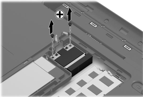
3. Remove the WLAN module by pulling the module away from the slot at an angle.
