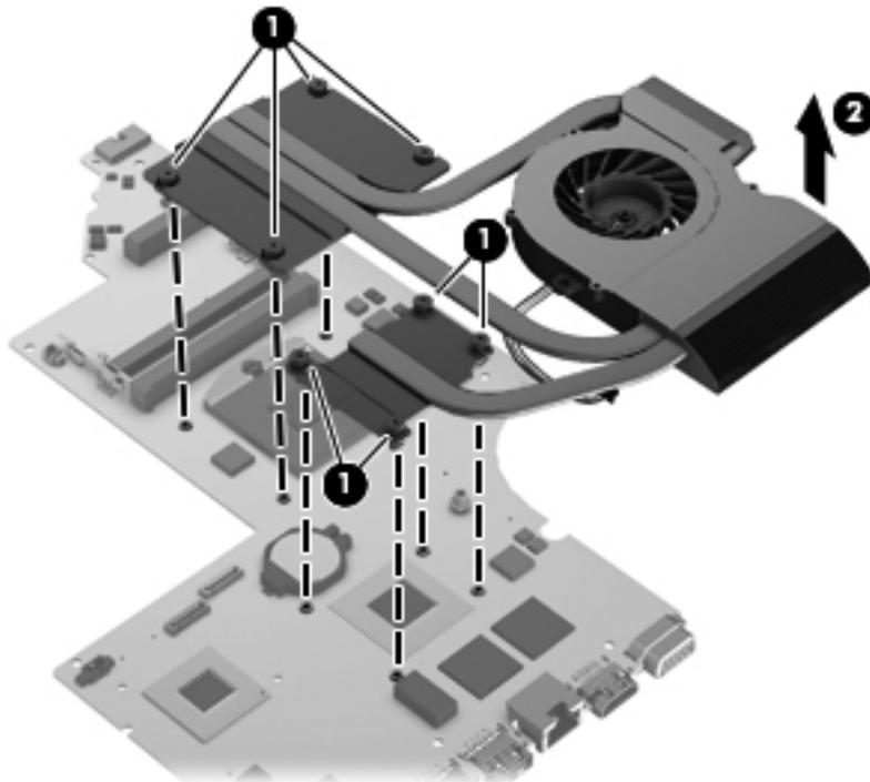
The thermal material must be thoroughly cleaned from the surfaces of the heat sink and the system board components each time the fan/heat sink assembly is removed. Replacement thermal material is included with the fan/heat sink assembly, processor, and system board spare part kits. Replacement thermal material is also available in the Thermal Material Kit.
