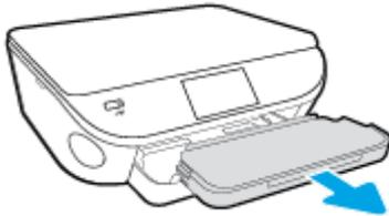
2. On the bottom of the output tray, move the output tray lock to the unlocked position, and then shift the release lever to release the tray extender.
