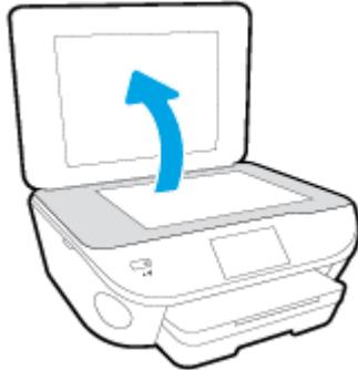
2. Load the original print side down on the right front corner of the glass.
