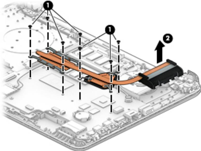
4. On models with UMA graphics, remove the four Phillips PM2.0×3.0 screws **(1)** on the heat sink that secure the heat sink assembly to the system board.
