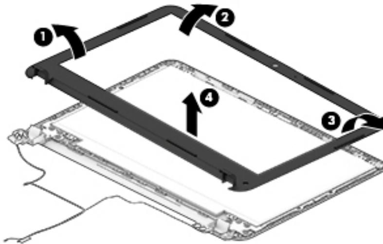
2. To remove the webcam/microphone module:
